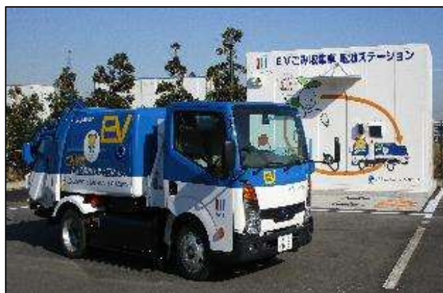
EV waste collection truck and charging station
