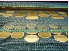
Conditioning for 24 hours with the temperature at  $21.5^{\circ}C \pm 1.5^{\circ}C$  and relative humidity at  $35\% \pm 5\%$ .
