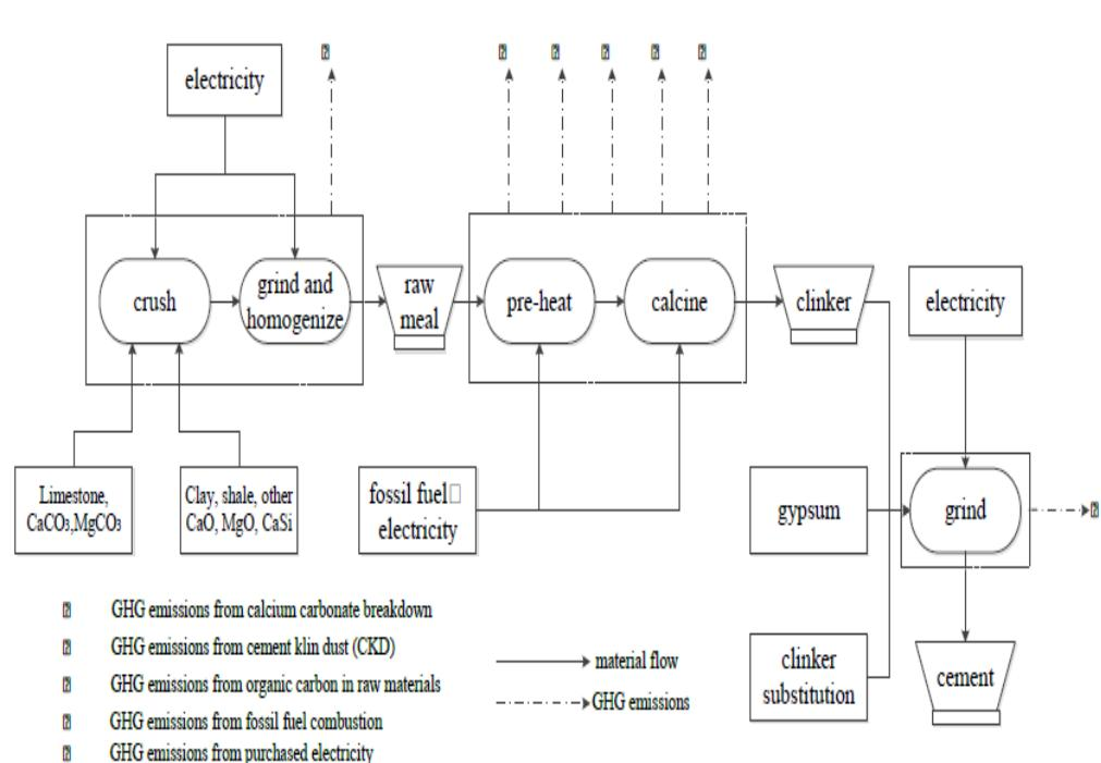
Figure 2 The overall flowchart of process for cement production
